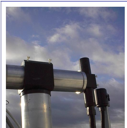
**Figure 2.7.1.1** *The tracker pointing the telescope measuring in zenith direction and the global irradiance cosine head (J1002) in the background to the right.*
