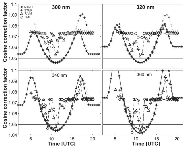
**Figure 2.7.3.3** Cosine correction factors for the Brewer #128, estimated for a day with complete cloud coverage for four wavelengths 300 (top left), 320 (top right), 340 (bottom left), and 360 nm (down right).
