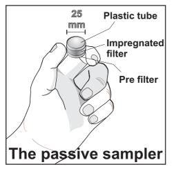
A sensitive diffusion sampler for sulphur dioxide (SO<sub>2</sub>) and nitrogen dioxide (NO<sub>2</sub>) in ambient air has been used in several investigations to undertake a screening of the spatial concentration distribution.
