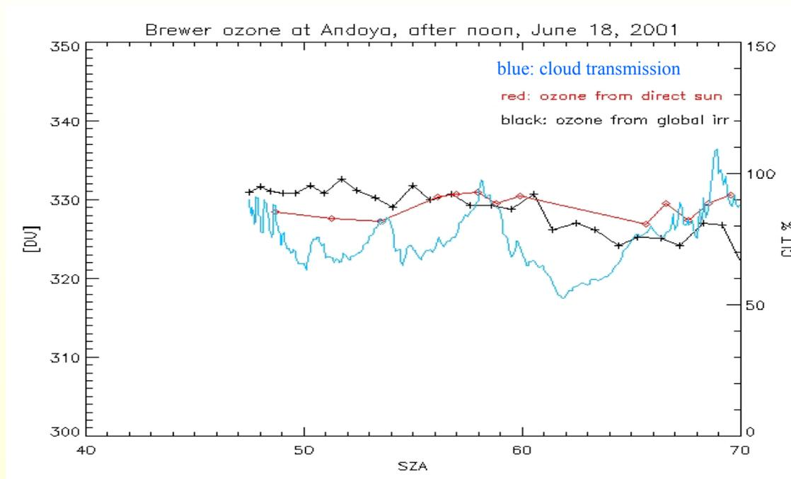
Global irradiance measurements are independent of direct sun (DS) and therefore important when cloudy conditions may prevent DS measurements. This will improve the measurement statistics for Andøya significantly
