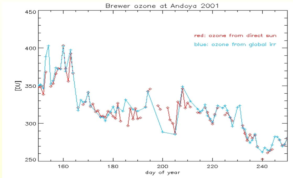
Further development of the analysis software for Brewer data allow us to calculate  $O_3$  not only from direct sun observations, but also from global irradiance measurements. The agreement of the ozone column derived from these two methods is good.
