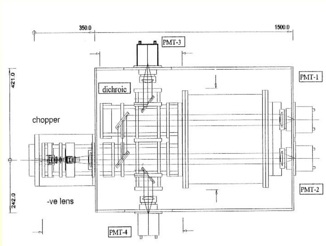
Drawing of the 2 channel daylight detection system (by Howermere Ltd., UK), based on capacitance-stabilised etalons (308 nm: single, 353 nm: double). During night time the light is divided into at the side mounted photomultipliers by-passing the etalon system.
