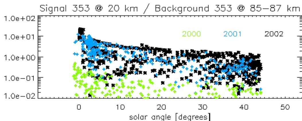
Signal-to-noise ratio for summer time (May - July) measurements in 2000, 2001 and 2002 as a function of solar elevation angle. An improvement since summer 2000 (green values) can be clearly seen. Additional efforts in 2002 led to better results in particular at high solar zenith angles.
