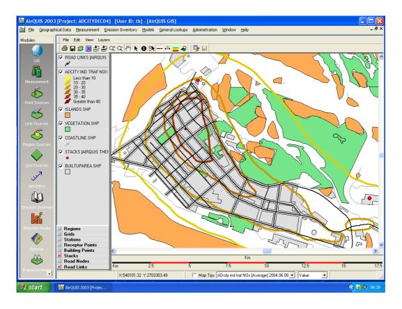
Figure 2: AirQUIS integrated GIS Module for presentation of modelling results.
