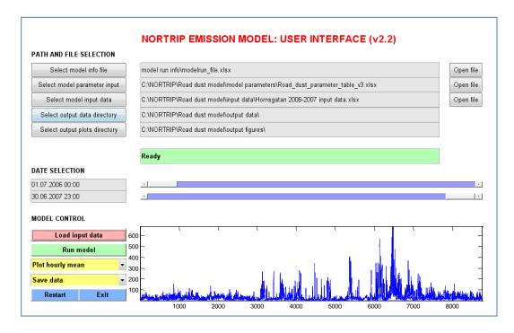
6. Once times have been selected the model can be run by pressing the 'Run model' button. The calculated concentrations will appear as red squares in the plot during the model run.
