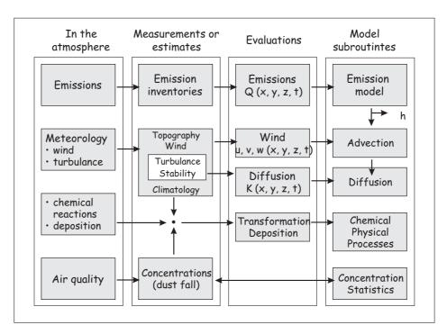
Figure 2: The procedure of an operational dispersion model used in practical applications.
