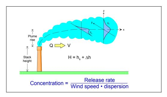
Figure 1: The concept of the Gaussian plume model.
