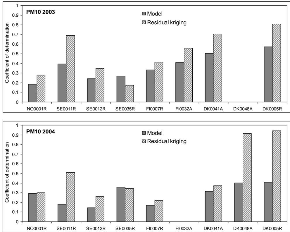
Figure 2.7. Daily mean coefficient of determination ( $R^2$ ) at the 9 Nordic stations for the years 2003 (top) and 2004 (bottom). Shown are the results from the Unified EMEP model and the residual kriging assimilation technique.
