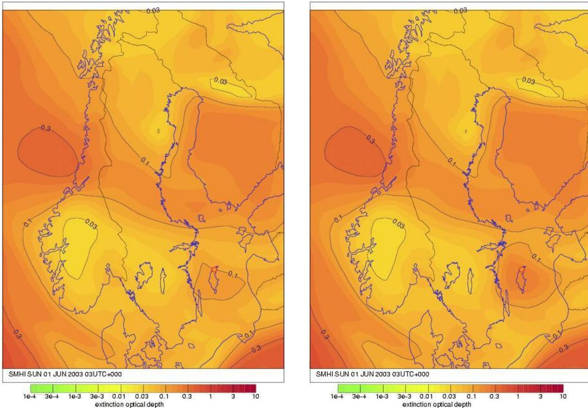
Figure 3.4. Aerosol optical depth computed from the MATCH photochemistry, sea salt, and PPM models (left), and data analysis result (right). Only one observation from the AERONET station on Gotland had been available for the analysis.
