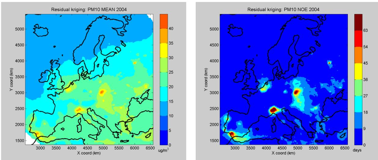
Figure 2.2. Maps showing the results of the residual kriging assimilation method for the 2 years 2003 (top) and 2004 (bottom). Shown are the annual mean  $PM_{10}$  concentrations (left), with a EU limit value of  $40 \mu g m^{-3}$ , and the number of exceedance days (right). The limit value for daily mean exceedance is  $50 \mu g m^{-3}$  and the maximum number of allowable exceedances of this value is  $36 \mu g m^{-3}$ .
