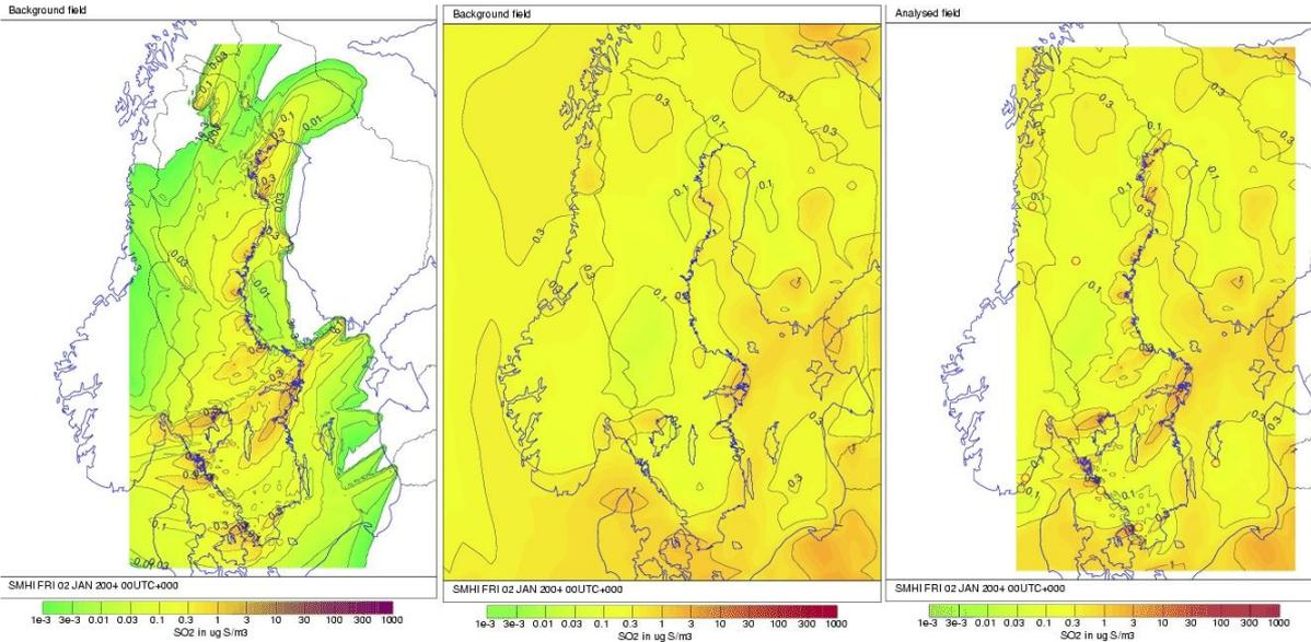
Figure 3.2.  $\text{SO}_2$  concentration field computed with the high-resolution MATCH-Sweden model (left), the low-resolution MATCH-Europe photochemistry model (middle), and the high-resolution 2dvar-analysis (right).
