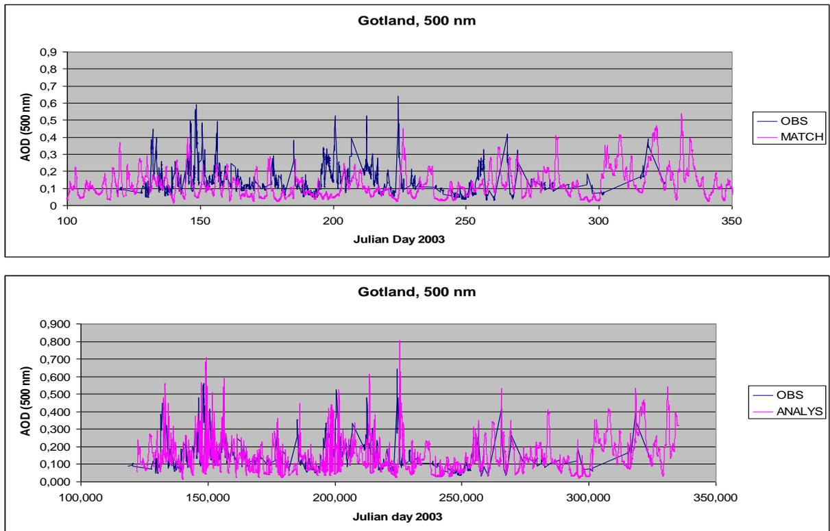
Figure 3.5: Upper panel: comparison of observed (blue) and modelled (pink) aerosol extinction optical depth at 500 nm on Gotland. Lower panel: Corresponding comparison of observations (blue) and data analysis results (pink). Note that the straight lines in the observation time series indicate data void regions. Thus the analysis relies on the background field during these periods.
