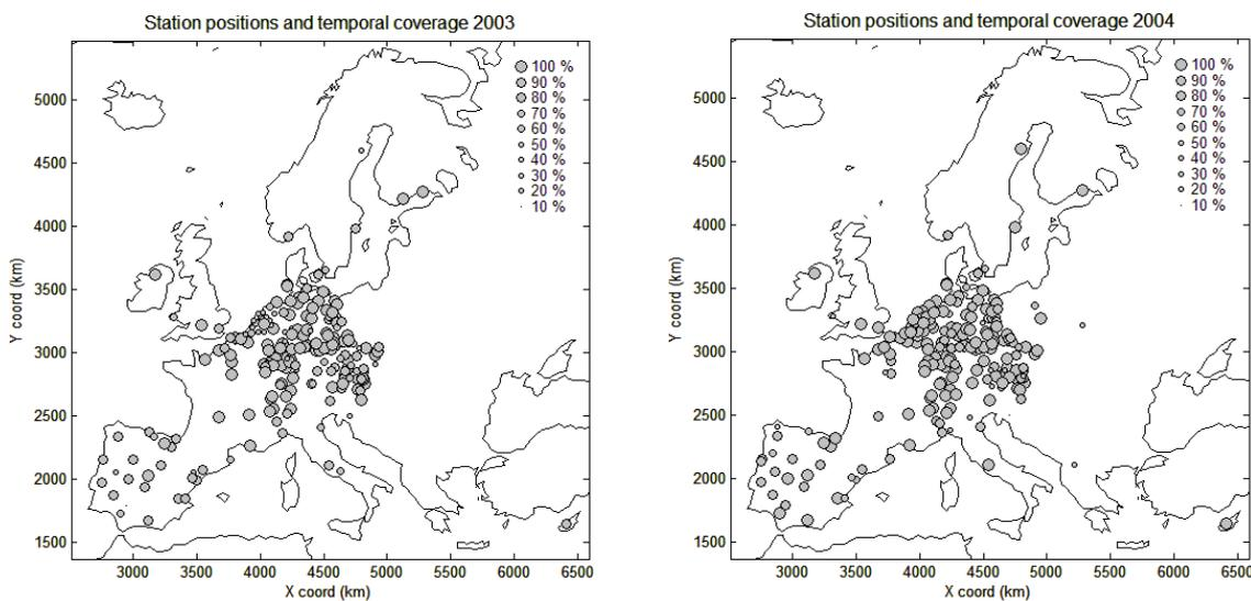
Figure 2.1. Positions and temporal coverage of the Airbase data used in the assimilations for the years 2003 (left) and 2004 (right). The size of the circles indicates the temporal coverage of the stations in %.
