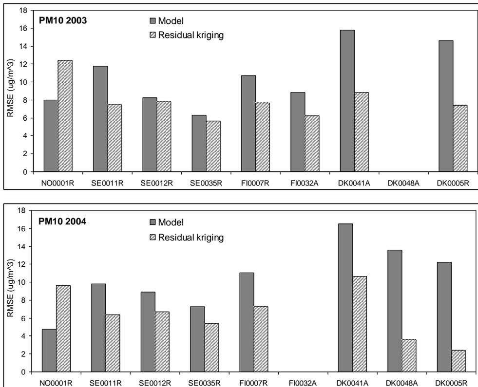
Figure 2.6. Daily mean RMSE at the 9 Nordic stations for the years 2003 (top) and 2004 (bottom). Shown are the results from the Unified EMEP model and the residual kriging assimilation technique.
