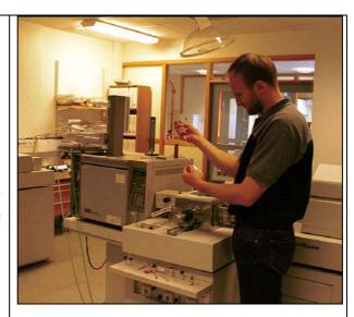
After extraction a volume of about 150 mL is reduced to 0.5 mL there are several reduction steps during a sample preparation. Before quantification the extract (ca. 20 mL) is reduced again to 0.2 mL. In general the volume reduction during the sample preparation process is about  $10\ 000\ x$ .
