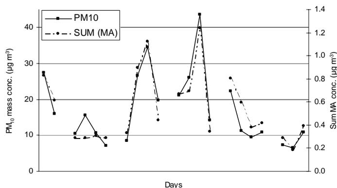
Figure 2:  $PM_{10}$  mass concentration and  $\Sigma$ MA concentration at Elverum during weekdays. Average temperature in the sampling period was  $-5.1^\circ\text{C}$  ( $-25.7 - 5.6$ ). The high degree of correlation indicates that wood burning is the dominating source.
