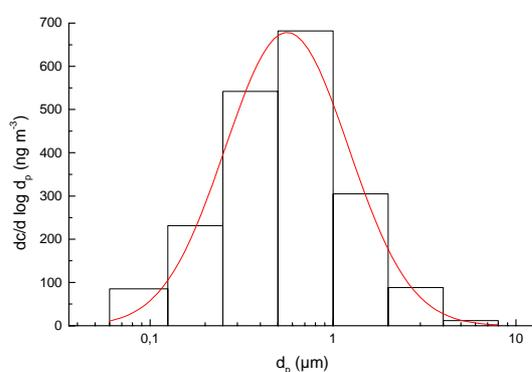
Figure 1: Particle size distribution of  $\Sigma$ MA measured in ambient air at Elverum, using a Berner cascade impactor. The line is the lognormal fit to the observed data given by bars. The mode diameter ( $x_c$ ) of the log normal distribution is 561 nm. 80% of the  $\Sigma$ MA is associated with particles  $< 1 \mu\text{m}$ .
