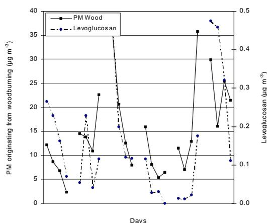
Figure 3: Comparison between levoglucosan and modeled concentrations of particulate matter due to wood burning contributing to the  $PM_{10}$  fraction on weekdays in Oslo. The discrepancies between the two datasets indicates that there are certain conditions that the model is not accounting for.  $R^2$  is 0.39 and  $r_p = 0.63$
