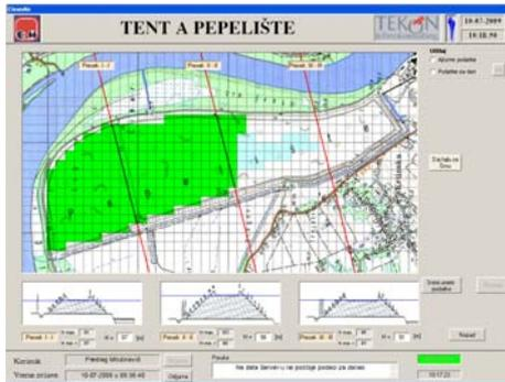
Fig. 4. Ash disposal site TNTA, dry 75% of active area white painted, blue pond
