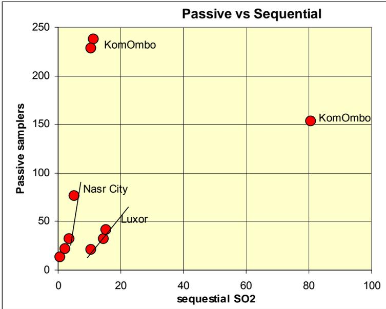
Figure 1: SO<sub>2</sub> concentrations measured by sequential samplers and by passive samplers during the same time periods.
