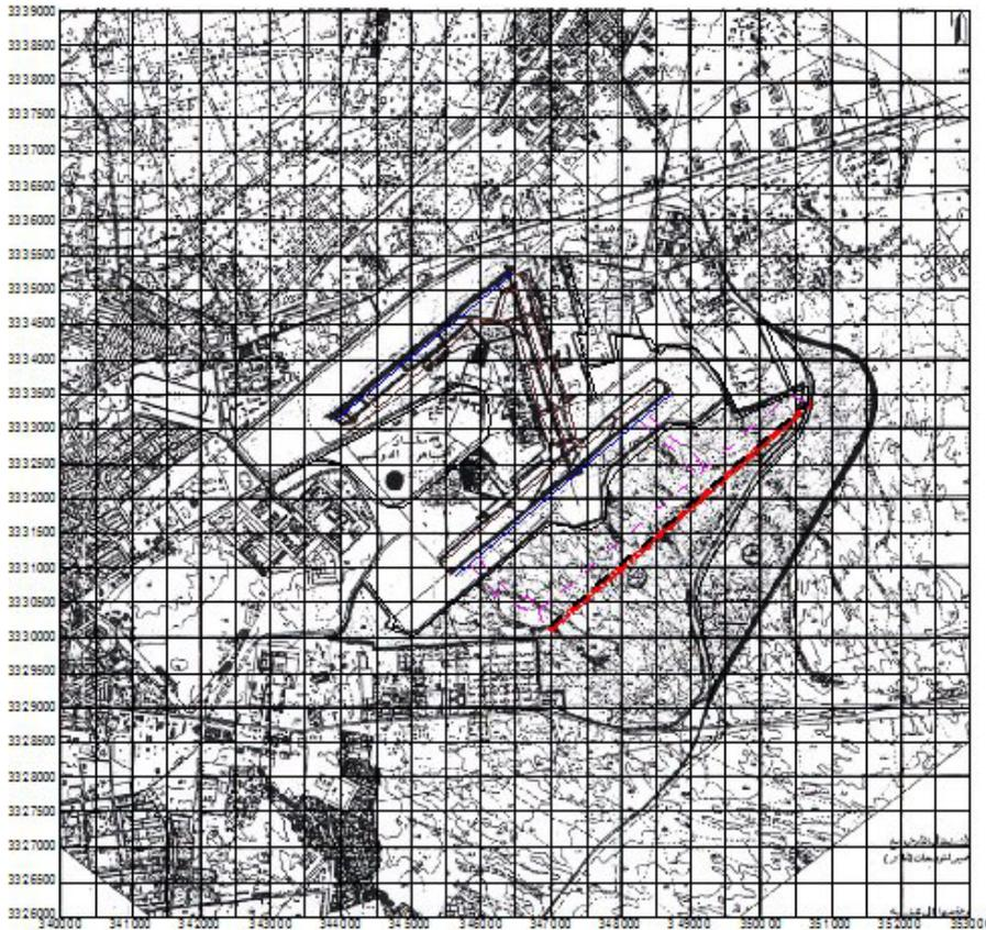
Figure 13: The modelling area and grids (500 m x 500 m) selected for the modelling of air pollution concentrations as a result of the airport activities.
