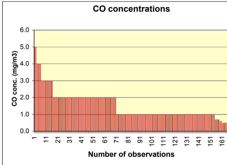
Figure 11: CO concentrations (hourly average) measured from 1 July to 8 July 2003.
