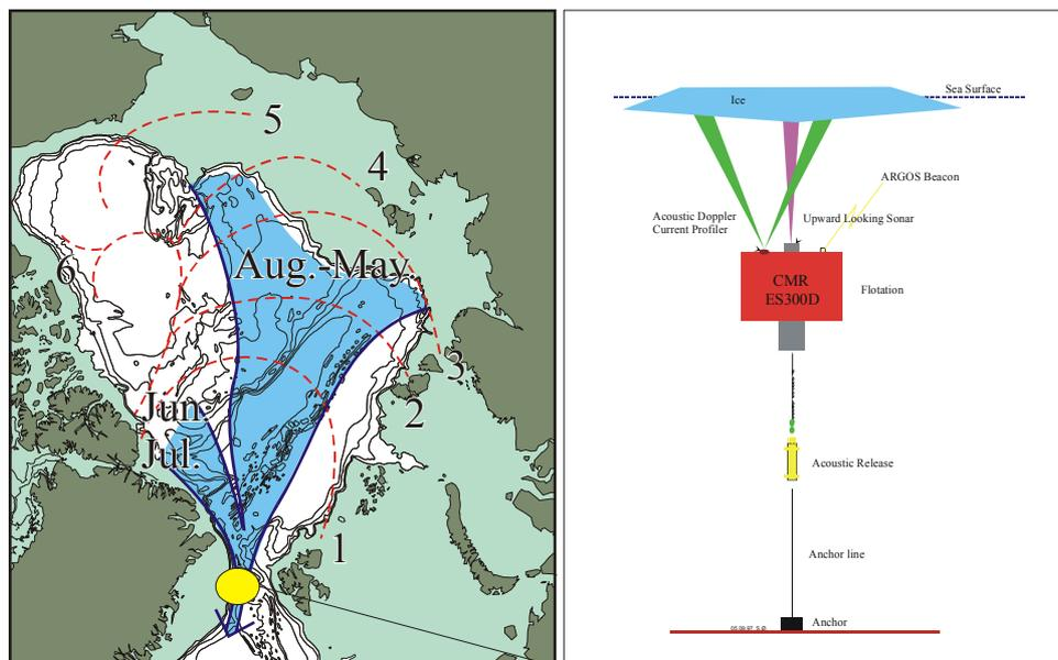
The ice and liquid freshwater in the Arctic Ocean is transported by the Transpolar Current through the Fram Strait. The yellow dot marks the monitoring position and the right a sketch of the mooring configuration
