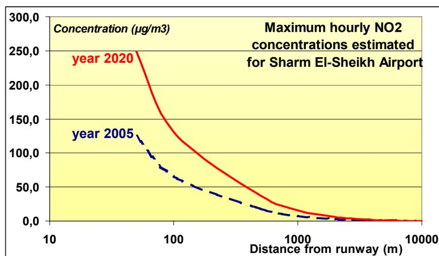
Figure 9: The estimated NO<sub>2</sub> concentration downwind from the runway at the Sharm El-Sheikh airport during peak hour traffic in 2005 and in 2020.
