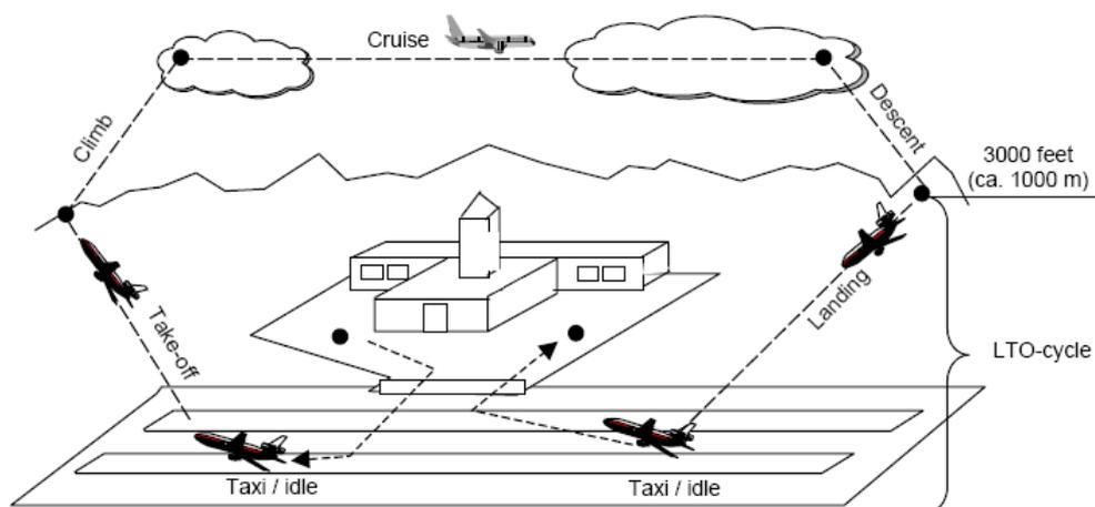
Figure 8: Aircraft operations divided into different cycles.
