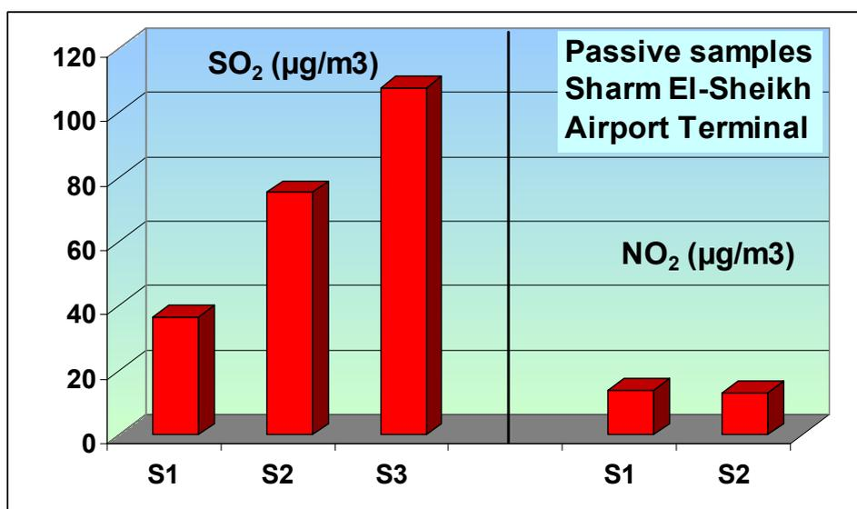
Figure 2: Passive samples of SO<sub>2</sub> and NO<sub>2</sub> collected at the Airport Terminal in Sharm El-Sheikh, from 23 Sep to 4 Oct 2003. S1 to S3 are sampling positions around the parking area of the Terminal building.
