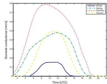
Fig. 5. Average diurnal cycles of stomatal conductance as predicted by the EMEP deposition module.
