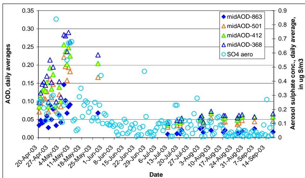
Figure 13. Daily AOD averages at 368, 412, 501, and 863 nm measured in Ny Ålesund, and daily averages of sulphate concentrations in airborne particles measured at the Zeppelin mountain station.
