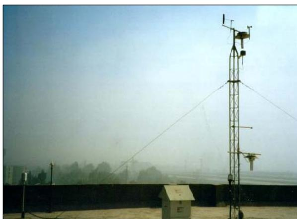
**Measurement Equipment** : Monitors for SO<sub>2</sub> and NO<sub>2</sub> , beta gauge for PM<sub>10</sub>, high volume sampler for TSP, dustfall collector and automatic weather station on 10-m mast.
