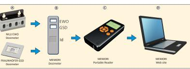
Fig. 1. The MEMORI Measurement Technology for Indoor Environments.
