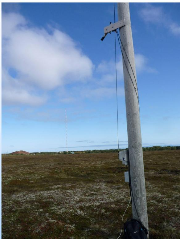
We used two autonomous TriOS Ramses hyper-spectral radiance sensors (radiance and irradiance) in order to measure the spectral radiances during the growing seasons March to end of October 2009-2012. TriOS sensor has a wavelength range of 320 - 950 nm. The radiance sensor measured the surface in an oblique off-nadir angle of 52° and the Field of View is 7°. The irradiance was measured with a hemispheric field of view.
