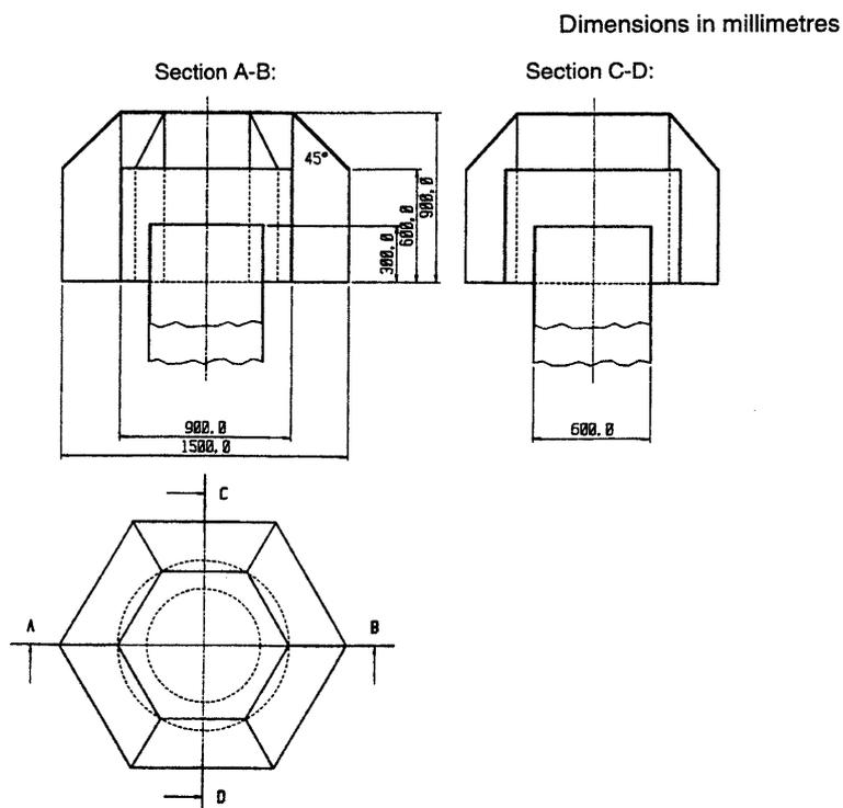
Figure 3: Design of WRAC inlet (CEN, 1998).
