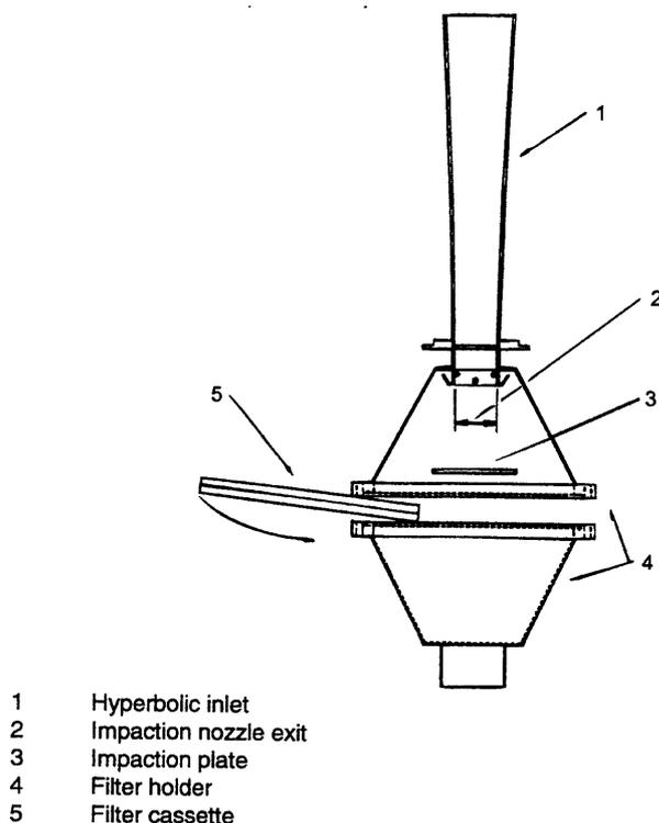
Figure 4: Design of WRAC  $PM_{10}$  stage (CEN, 1998).
