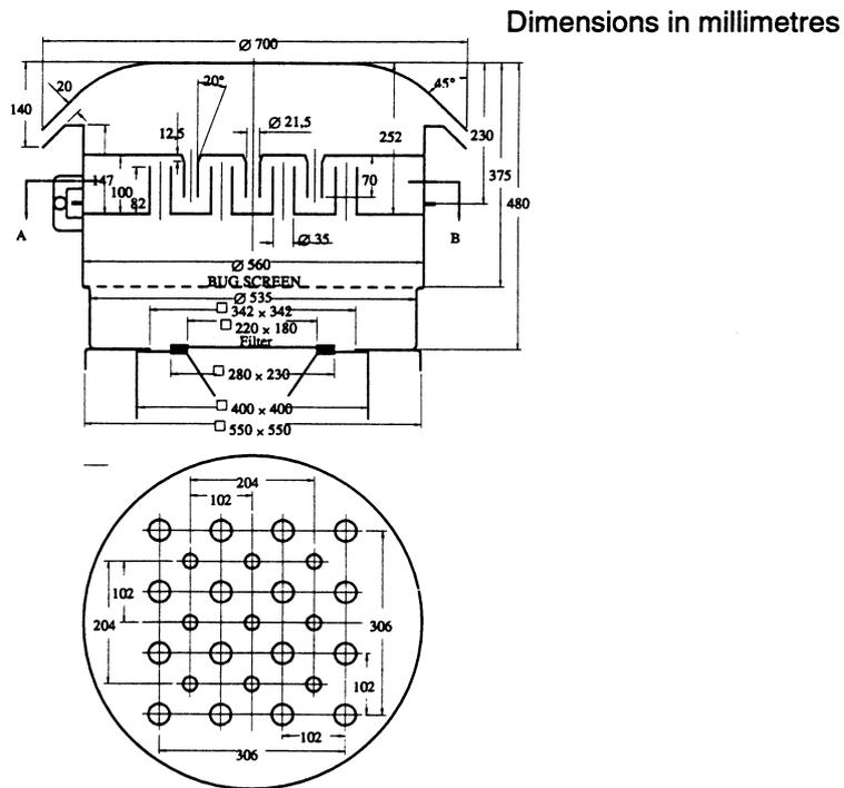
Figure 2: Design of 68 m<sup>3</sup>/h HVS-PM<sub>10</sub> sampling inlet (CEN, 1998).
