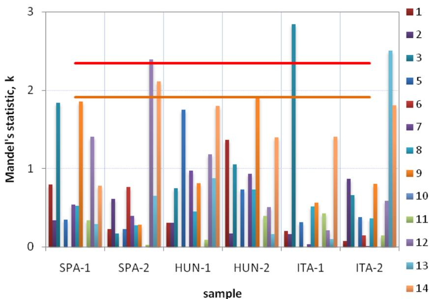
Figure 5.5: Mandel's  $k$  statistic values for between-laboratory consistency on EC/TC ratio obtained from the entire database, grouped by laboratory (panel a) and by sample (panel b). For 11 laboratories  $k$  and two replicates values should be  $< 2.34$  at 1% significance level (red line) and  $< 1.91$  at 5% significance level (orange line).
