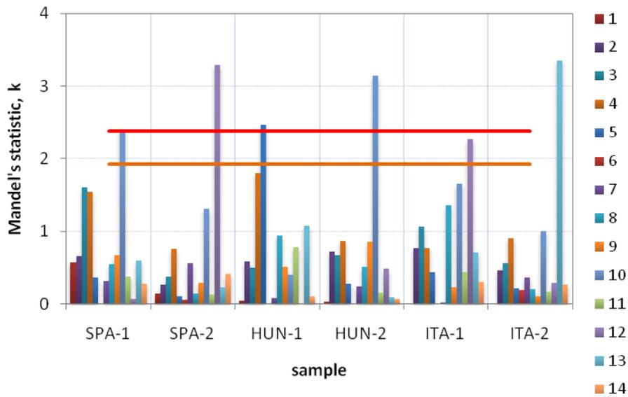
Figure 5.3: Mandel's  $k$  statistic values for between-laboratory consistency on TC data, grouped by laboratory (panel a) and by sample (panel b). For 13 laboratories and 2 replicates,  $k$  values should be  $< 2.38$  at 1% significance level (red line) and  $< 1.92$  at 5% significance level (orange line).
