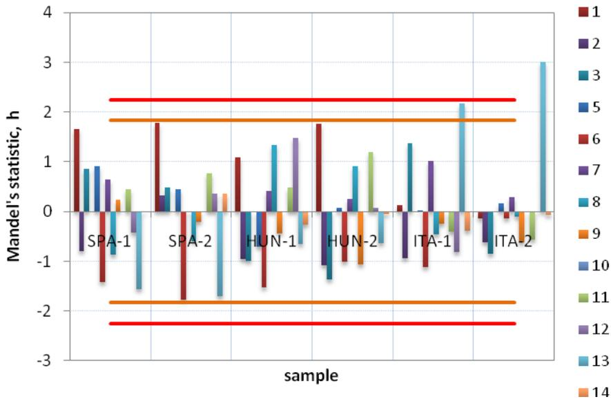
Figure 5.4: Mandel's  $h$  statistic values for between-laboratory consistency on EC/TC ratios obtained from the entire database, grouped by laboratory (panel a) and by sample (panel b). For 12 laboratories  $h$  values should be  $< 2.25$  at 1% significance level (red line) and  $< 1.83$  at 5% significance level (orange line).
