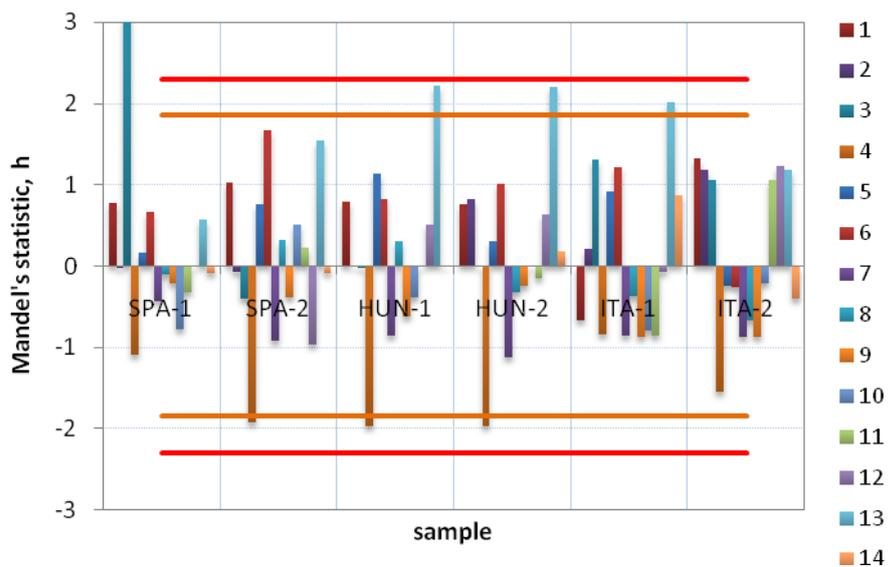
Figure 5.2: Mandel's  $h$  statistic values for between-laboratory consistency on TC data, grouped by laboratory (panel a) and by sample (panel b). For 14 laboratories,  $h$  values should be  $< 2.30$  at 1% significance level (red line) and  $< 1.85$  at 5% significance level (orange line).
