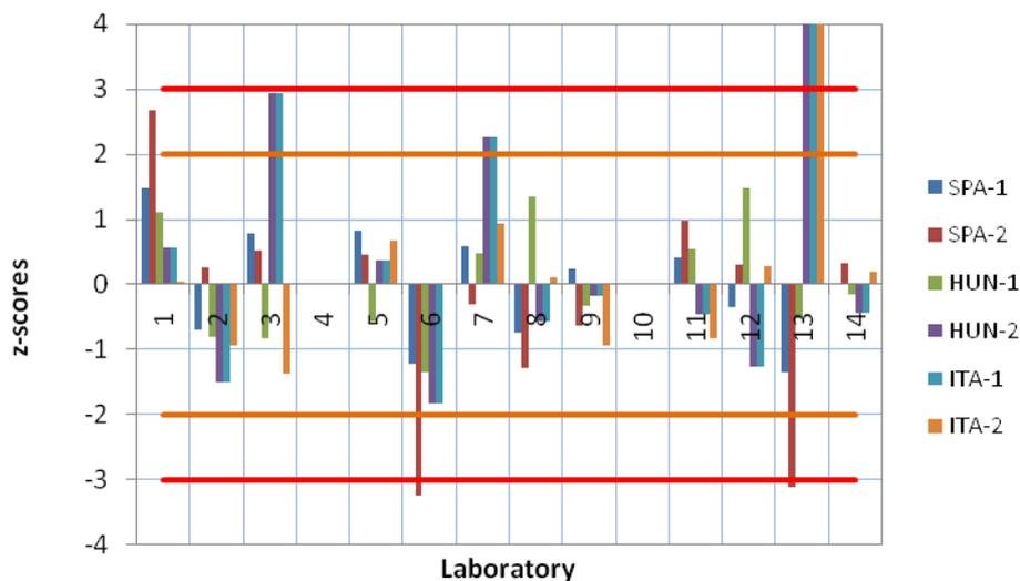
Figure 5.7: z-scores for EC/TC ratios calculated using  $\sigma^*_a$  from data obtained in a round of a proficiency testing scheme.
