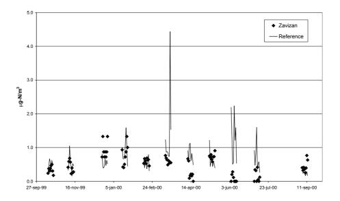
*Figure 2: Comparison of measurements at Zavizan with reference sampler; results for nitrogen dioxide.*
