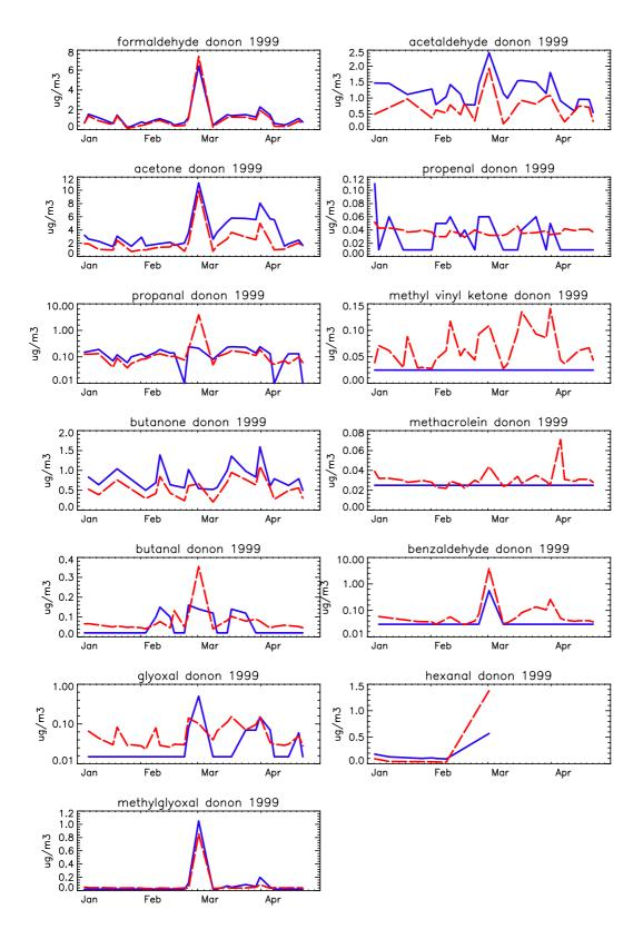
*Figure 8:* Results of parallel sampling and analyses of carbonyl compounds at Donon by NILU (blue full line) and EMD (red dashed line) in January–April 1999. Note the logarithmic axis for propanal, benzaldehyde and glyoxal (due to outliers for these compounds).
