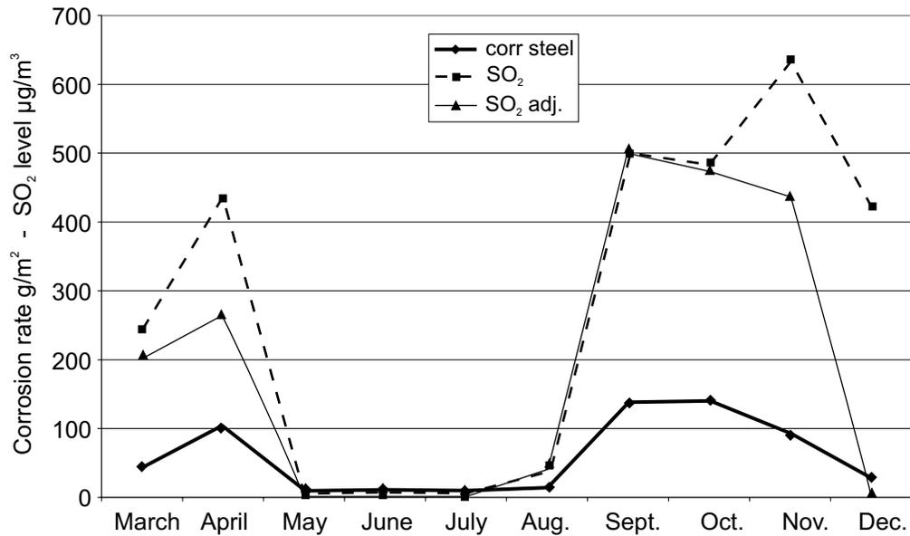
**Figure 2 - Plot of monthly steel corrosion in g/m<sup>2</sup> together with the monthly SO<sub>2</sub> values and the “effective” SO<sub>2</sub> values using -4°C as the limit for corrosion**
