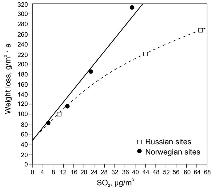
**Figure 3 - Annual loss of carbon steel versus annual average sulphur dioxide concentration along the Norwegian – Russian border**
