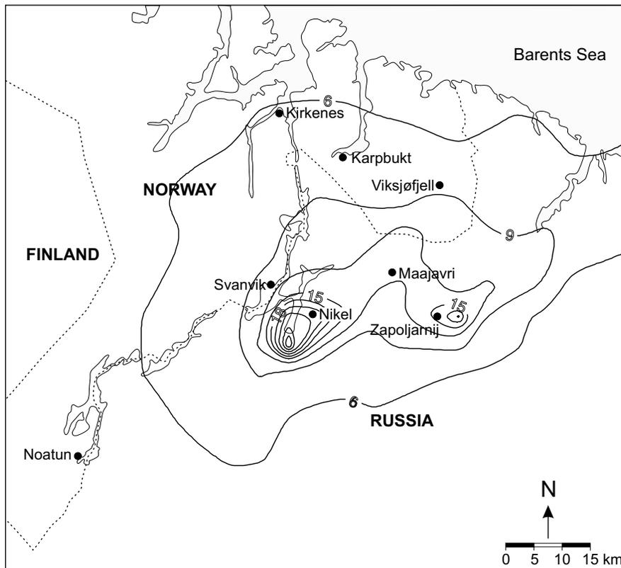
**Figure 6 - Map of the first year of corrosion for zinc inside a modelling area of 110x100 km along the Norwegian – Russian border (corrosion in  $\text{g/m}^2 \cdot \text{year}$ ).**
