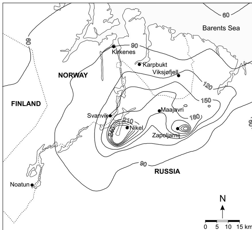
**Figure 5 - Map of the first year of corrosion for steel inside a modelling area of 110x100km along the Norwegian – Russian border (corrosion in g/m<sup>2</sup>•year).**
