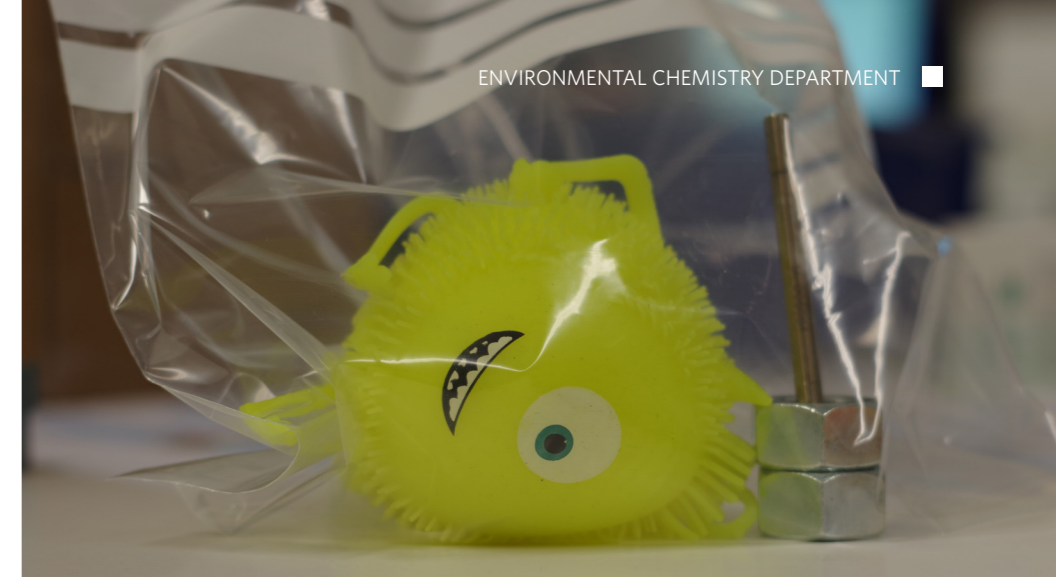
This image shows one of the toys included in the study in an airtight ziplock bag. The metal tube is the Tenax TA air sampler. Photo: Ingunn Trones, NILU.
