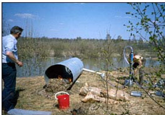
Figure 1. The experimental layout of measuring emissions from bonfires and burning of rubbish (NILU, 2003).
