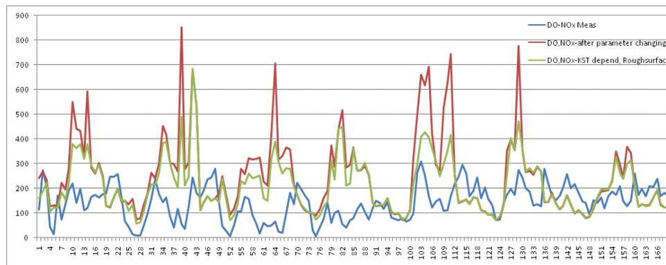
Figure 11: Model estimated NOx concentrations at Doste using new dispersion parameters for rough surface conditions (green curve) and old dispersion (red curve) versus measured concentrations (blue line) at the Doste station for February 2007. (Test date 23 Oct 2007).
