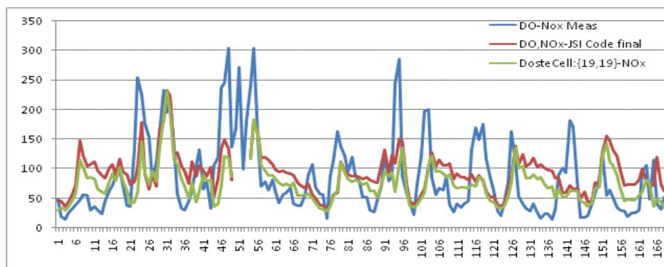
*Figure 14: Model estimated NOx concentrations at Doste using final input data concerning boundary layer parameterisation and model layers (Hiway2) (red curve) versus measured concentrations (blue line). The green line shows the model estimated average km-scale grid cell concentrations.
