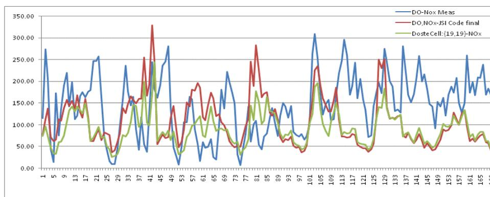
*Figure 13: Model estimated NO<sub>x</sub> concentrations at Doste using final input data concerning boundary layer parameterisation and model layers (Hiway2) (red curve) versus measured concentrations (blue line). The green line shows the model estimated average km-scale grid cell concentrations.*
