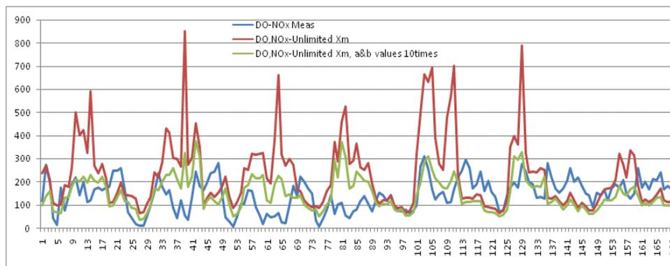
Figure 10: Model estimated NOx concentrations at Doste using a strongly enhanced dispersion (green curve) and old dispersion (red curve) versus measured concentrations (blue line) at the Doste station for February 2007. (Test date 11 Oct 2007).
