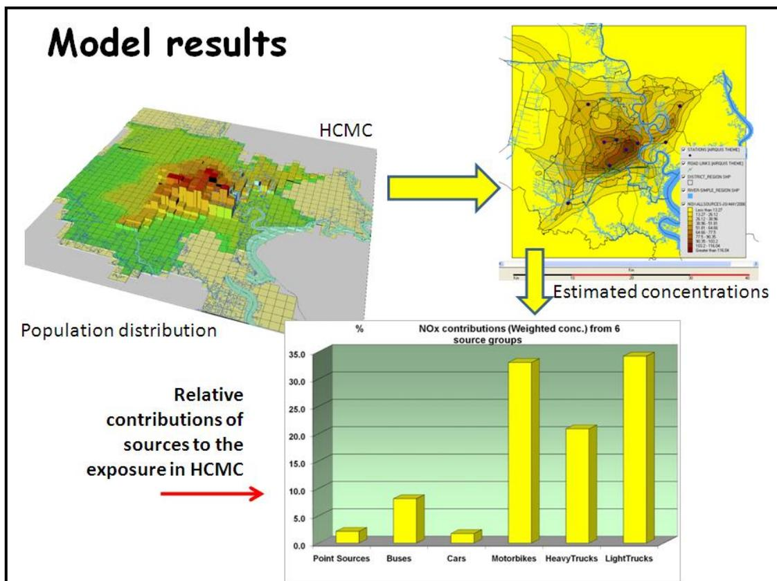
Figure 16: Population distribution and NOx concentration distributions from model estimates represented the input for estimating the relative contributions of sources to the exposure of NOx in HCMC.
