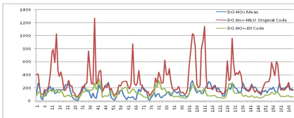
*Figure 12: Model estimated NOx concentrations at the Doste site using new dispersion parameters based on drag wind speeds (Hiway2) (green curve) and old dispersion (red curve) versus measured concentrations (blue line).*
