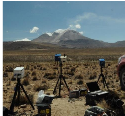
Fig. 2: Photo from the measurement site showing 2 UV SO 2 cameras (blue), the DOAS instrument and an IR SO 2 camera (white, left side).
